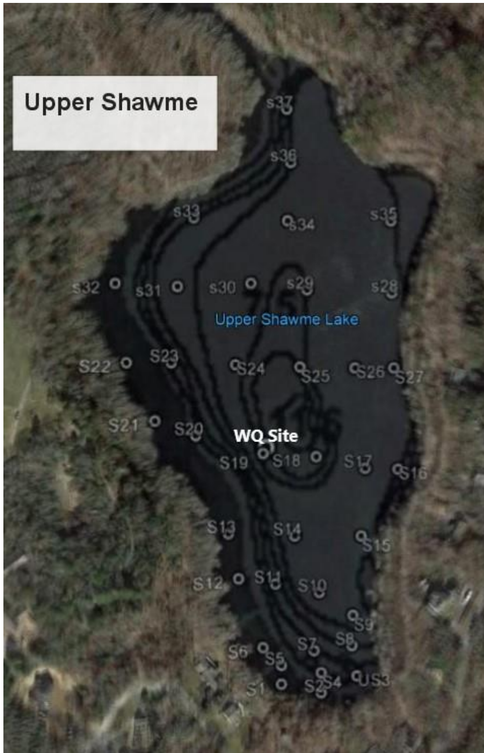
Figure 5. Upper Shawme Pond survey points with bathymetry.
