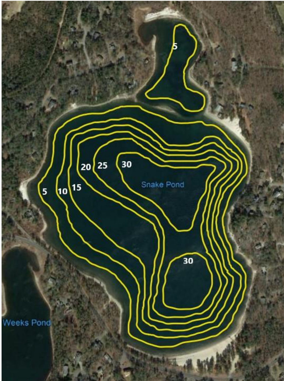
Figure 37. Bathymetry of Snake Pond from WRS 2018 measurements.
