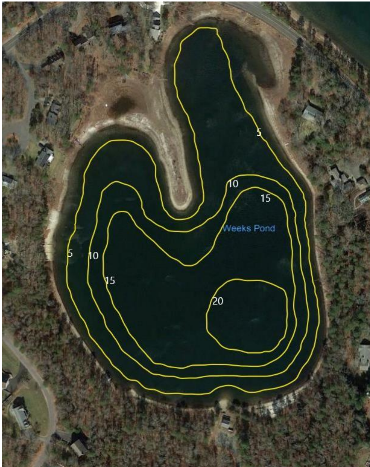
Figure 41. Bathymetry of Weeks Pond from WRS 2018 measurements.
