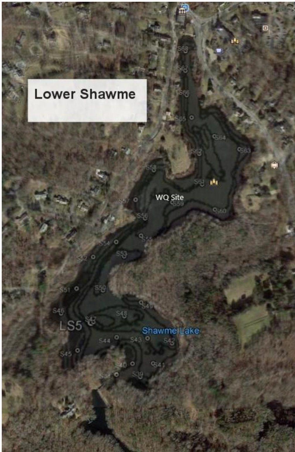
Figure 7. Lower Shawme Pond survey points with bathymetry.
